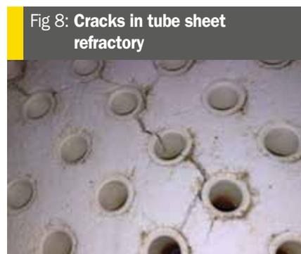
Fig 8: Cracks in tube sheet refractory
