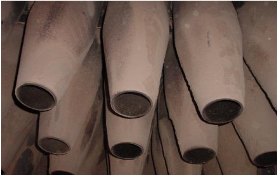
Figure 3: These OXYTRON ceramic cones have been in use for more than 12 years and show no signs of wear or wall degradation.
