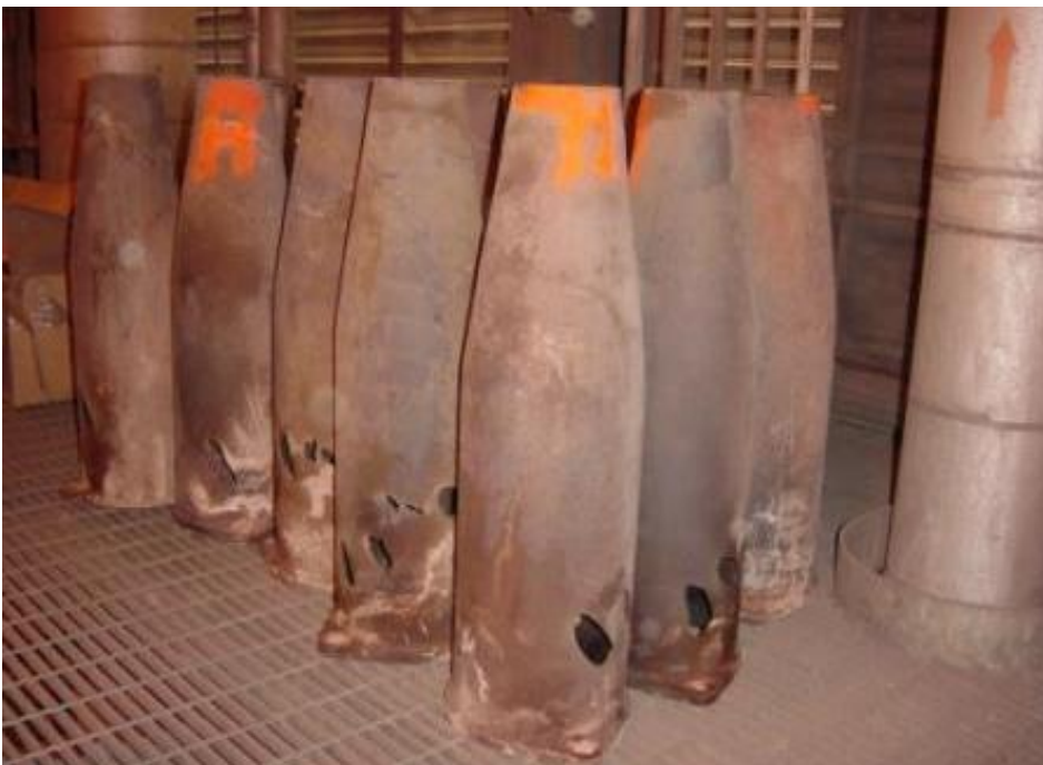
Figure 2: These metal cones removed from a mechanical dust collector show typical failure areas caused by dust laden gases eroding the metal.
