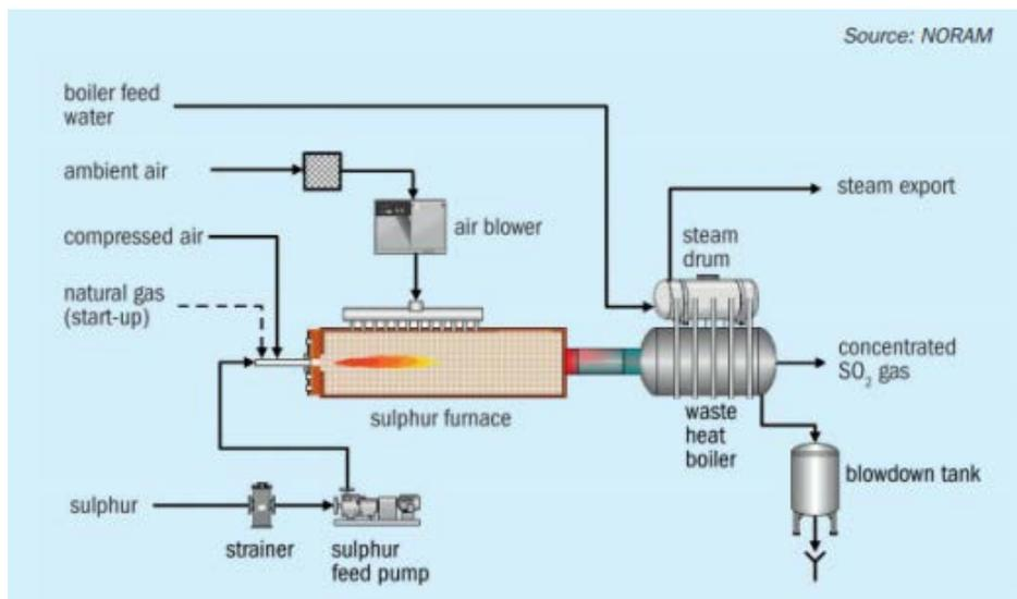
Figure 10: NORAM-Cellchem SO<sub>2</sub> production system with an SF burner and heat recovery system
