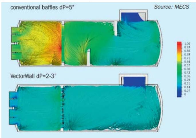
Figure 6: Pressure drop for 3 baffle walls vs 1 VectorWall
