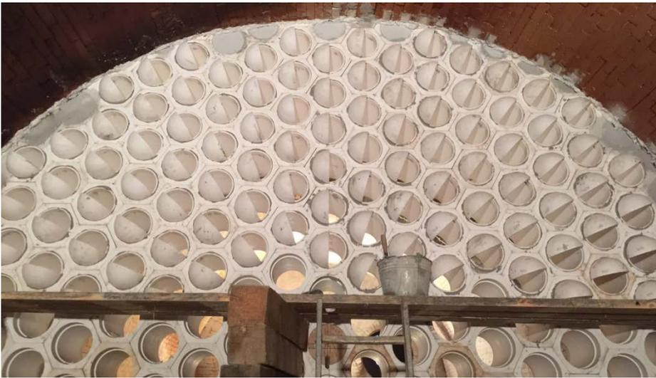
**Figure 8:** Recent VectorWall installation for narrower residence time distribution
