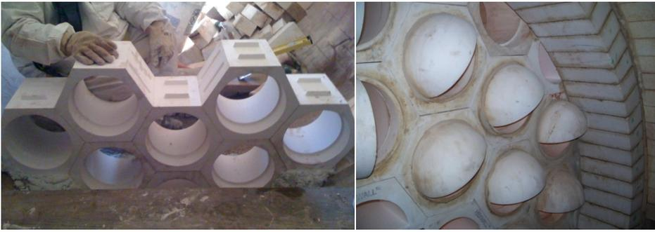
Figure 5: MECS® VectorWall ceramic furnace internals
