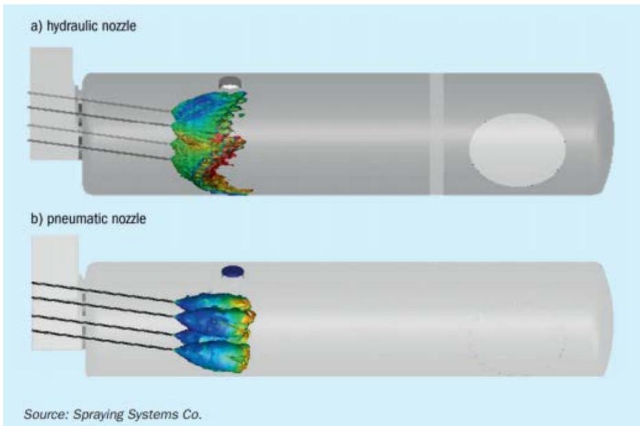
**Figure 1:** Cross section of furnace and spray coverage for different nozzle types
