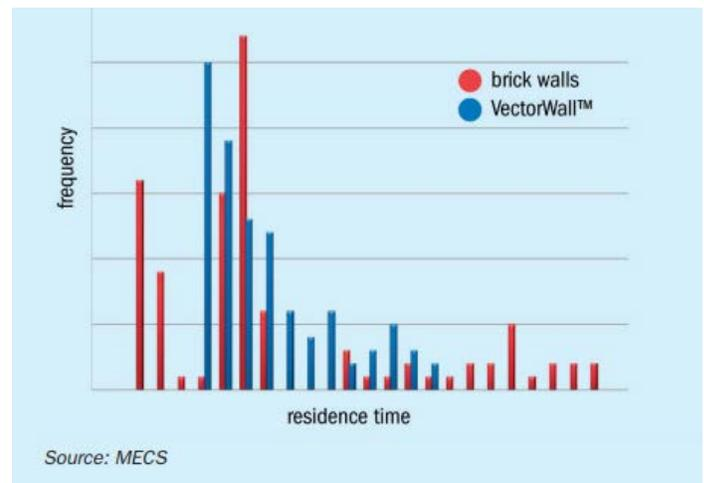
Figure 7: Residence time for 3 baffle walls vs 1 VectorWall
