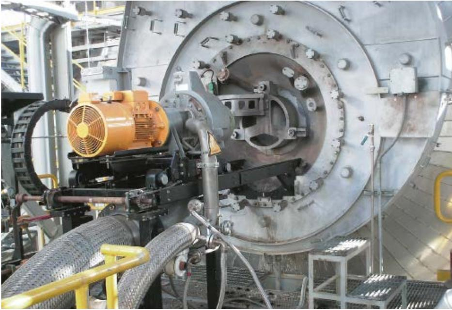
**Figure 12:** Outotec® LURO2 sulphur burning system
