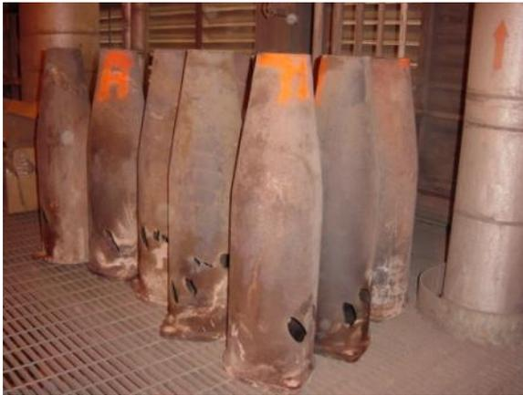
**Figure 4:** These metal cones removed from a mechanical dust collector show typical failure areas caused by as-laden gases eroding the metal.
