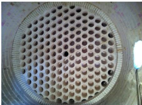
**Figure 4:** VectorWall at Bern Gas Plant
