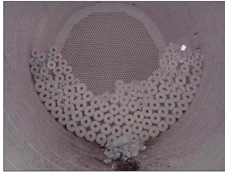
**Figure 2:** Cylindrical shape conventional checker wall
