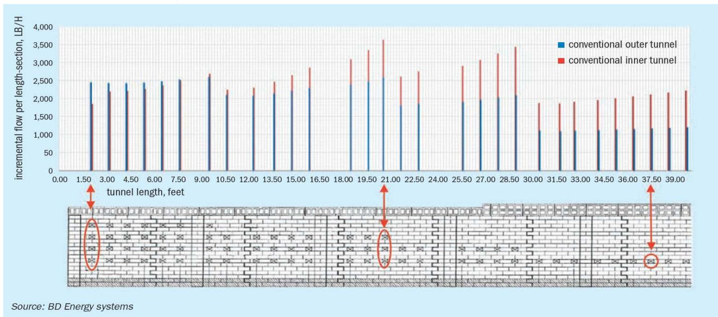
**Figure 9:** Incremental flow per open-area column for conventional inner and outer tunnels
