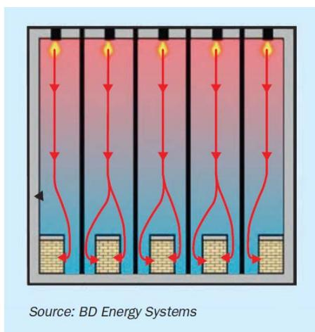
Figure 8: Flue gas flow into radiant box tunnels
