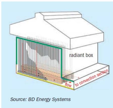
Figure 7: Radiant box flue gas flow
